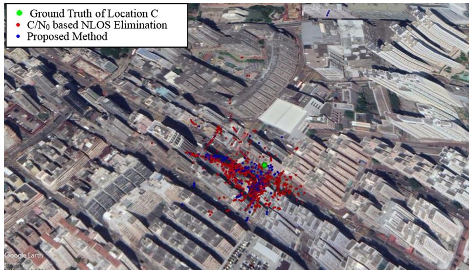
Fig. 13. Positioning results based on the elimination of the NLOS signals detected from the proposed GBDT with multi-feature-based method and single C/N_0 based method in Location C.
